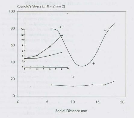
**Fig. 6** Radial profile of Reynold's stress at an agitation speed of 2.5 r/s for medium without FBS (+) and with 10% FBS (.)
