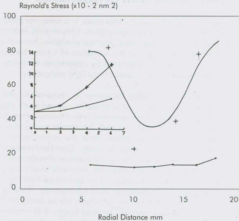
**Fig. 6** Radial profile of Reynold's stress at an agitation speed of 2.5 r/s for medium without FBS (+) and with 10% FBS (.)
