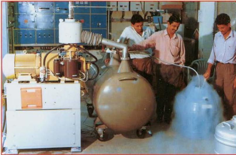
Liquid nitrogen plant was installed in the basement of Jidnyasa building. I & M staff are all smiles at the first flow of liquid nitrogen.
